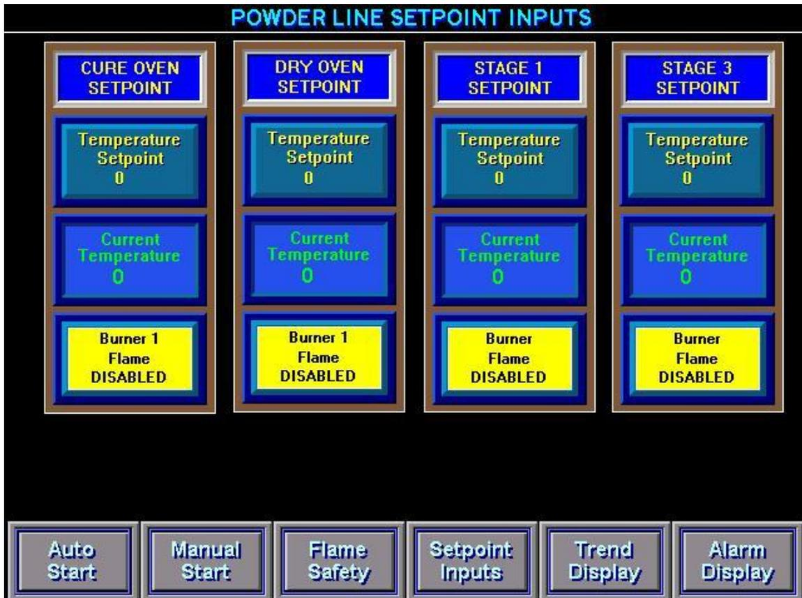
A new Temperature Setpoint Can be entered by depressing any of the Oven or Washer Temperature Setpoint buttons above the Current Setpoint Temperature.
