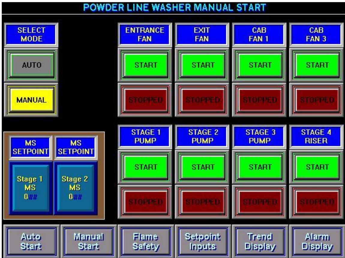
All components must be in **Manual Mode** to be started Manually. If **Manual** is not displayed in the box on the right of the screen then it must be toggled from the **Auto** to **Manual**.
